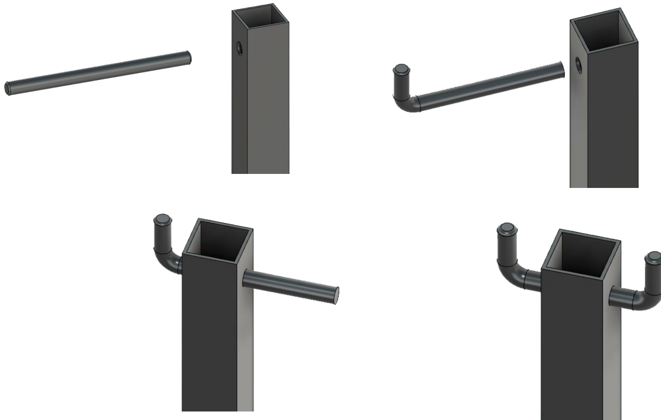
Process of insertion of Bent rod
